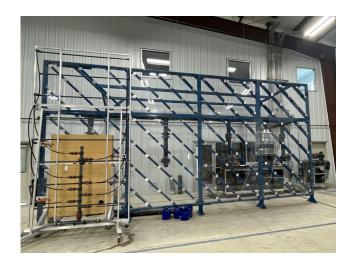
**NAFS:** The industry standard for testing and rating fenestration products for air, water, and structural performance. ACT's state of the art test wall and console provide quick and accurate test results. Pictured is our 24' x 12' tall test wall.
