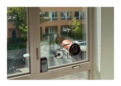
ASTM E576 is a test used to measure the frost or dew point inside sealed insulating glass units (IGU). IGU's are hermetically sealed to prevent air and moisture from entering the sealed cavity. Desiccants are placed inside the IGU to remove incidental moisture trapped during fabrication. This test verifies if moisture has penetrated the IGU and overwhelmed the desiccants, causing premature failure.
