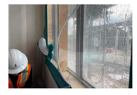
ASTM E1105 is a comprehensive test used to evaluate the water resistance of installed windows, doors, skylights, and curtain walls, by simulating heavy rain conditions. This test helps ensure the durability and performance of these assemblies.
