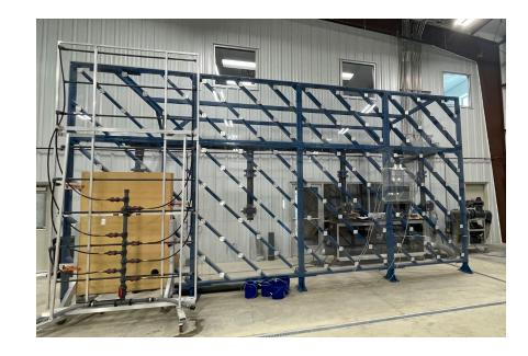
ASTM E283 Air Infiltration Testing measures air leakage through windows, doors, and building envelope components. This test is vital for ensuring energy efficiency, verifying compliance with energy codes, and enhancing occupant comfort. By identifying air leaks, you can help clients reduce heating and cooling costs while providing confidence in the quality and efficiency of your products.
